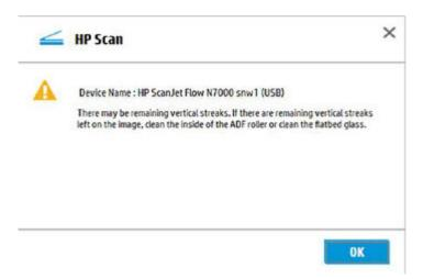
If any vertical streaks are seen on the image after this operation, either clean the flatbed glass or clean the roller on the inside of the Automatic Document Feeder (ADF), depending on the product type.
